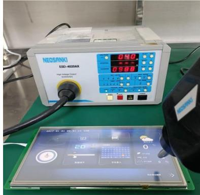
3.1 Electrostatic discharge test
